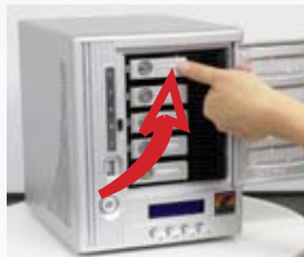
Step 2- Secure Canister Latches
