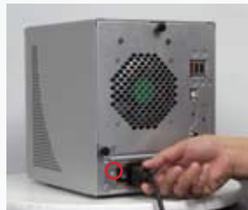
Step 3- Connect Power and turn on switch
