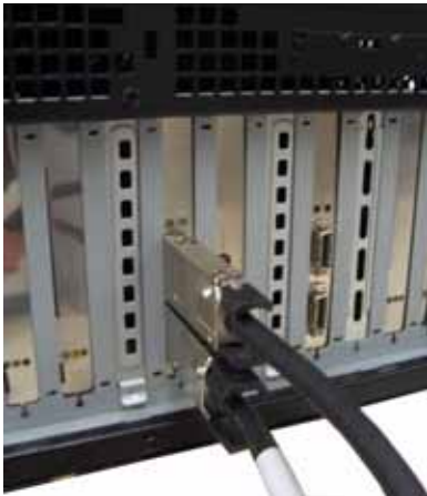
Figure 2-6 DSE4XM with Four x4 Connections
