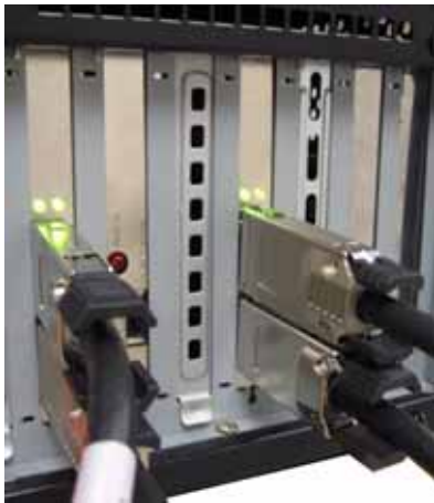
Figure 2-6 DSE4XM with Four x4 Connections
