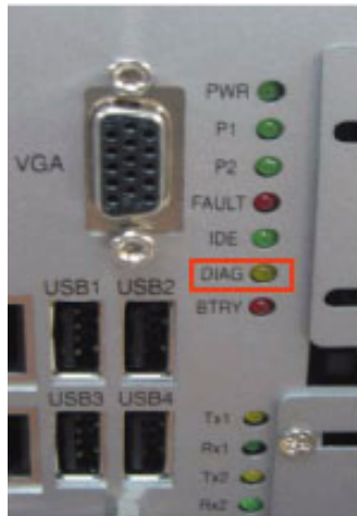
Figure 2.13: LED Location for System Diagnosis
