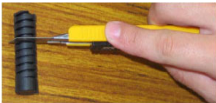
Figure 3.4: Adjust the Anti-Vibration Rubber
