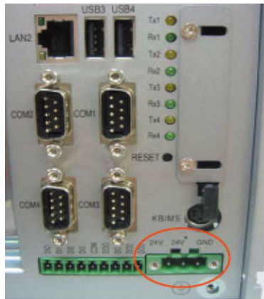
Figure 2.11: Location of Power P1 and P2
