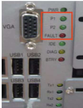
Figure 2.12: LED Locations to Monitor Power Input
