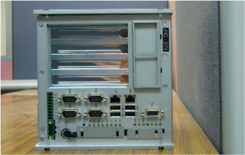
Figure 3.6: UNO-3074 Improper Installation (1)
