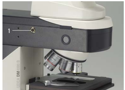
Fig. 11 Objective turret with labeled objective receptacles
