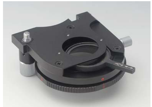
Fig. 29 Inserting the polarizer 1 The plug cap is replaced with the polarizer.
