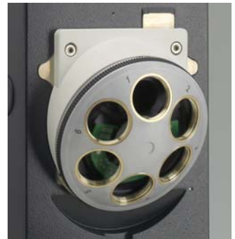
Fig. 11 Objective turret with labeled objective receptacles
