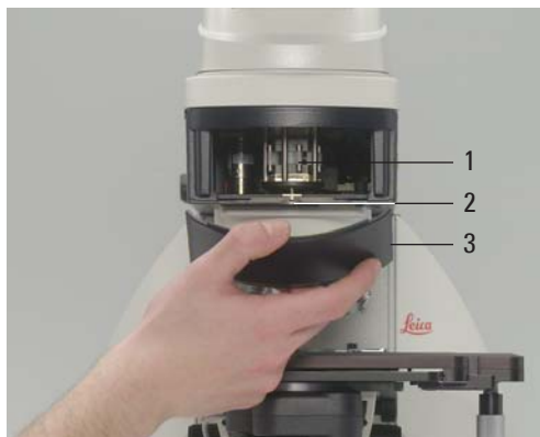
Fig. 26 Inserting the filter or reflector cubes
