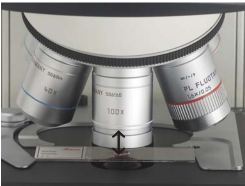
Fig. 63 Immersion objective (released)
