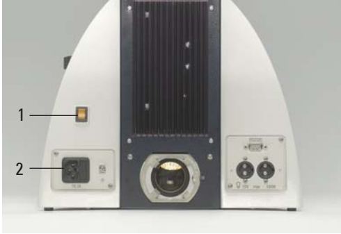
Fig. 35 Rear side of electronics box CTR5000
