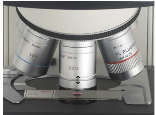
Fig. 64 Immersion objective (locked)
