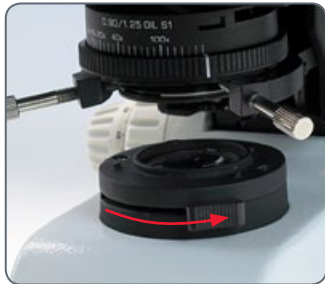
Close the Koehler field diaphragm
