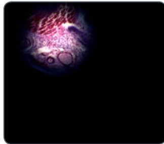
Close the Koehler field diaphragm
