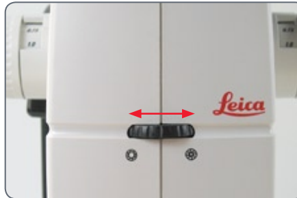
Adjusting the double-iris diaphragm using the knurled ring
