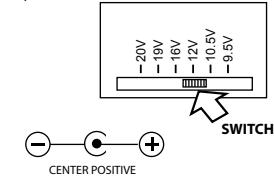
Use the diagram shown above to verify that your laptop uses "center positive" polarity as most all laptops use "center positive" polarity. Do not use the LAC50 if your laptop shows "center negative" polarity.
