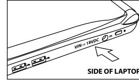
2.) Review the power ID plate on the bottom of the laptop to be powered. Look for the word "DC RATING or INPUT" followed by a number and VDC.
