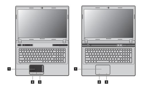
Touchpad To move the cursor on the screen, slide your fingertip over the pad in the direction in which you want the cursor to move.
