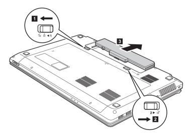
**4** Install a fully charged battery.
