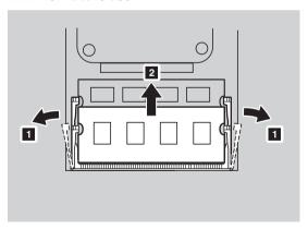
• Align the notch of the DDR3 SDRAM with the protrusion of the socket and gently insert the DDR3 SDRAM into the socket at a 30-45° angle.
