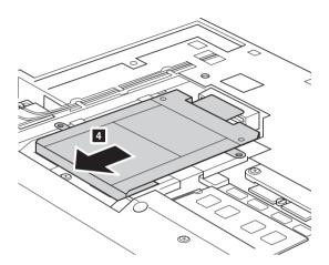
Take out the hard disk drive secured in a metal frame 5.
