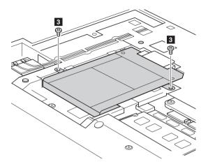
6 Pull the HDD bracket in the direction shown by arrow 4.
