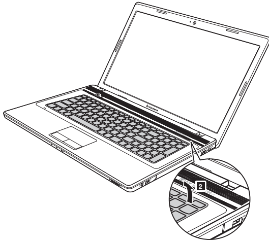
Figure 8. Removal steps of keyboard (continued)
