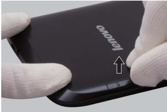
Figure 2. Removal steps of Micro SD card
