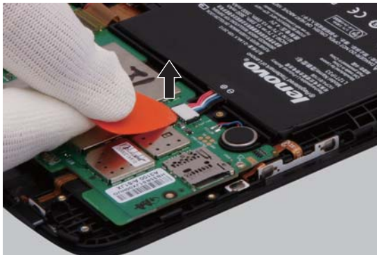
Figure 6. Removal steps of battery pack
