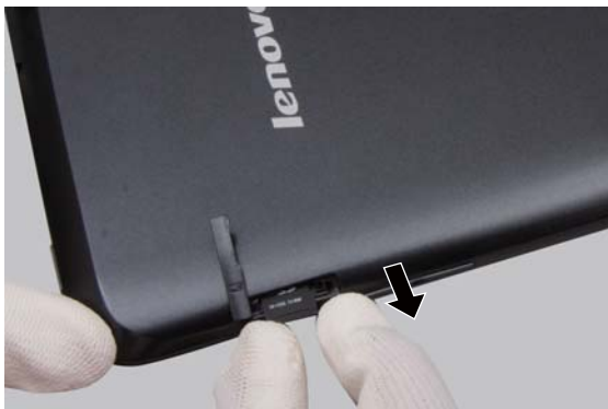
Figure 2. Removal steps of Micro SD card (continued)
