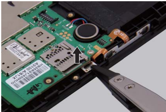
Figure 8. Removal steps of system board
