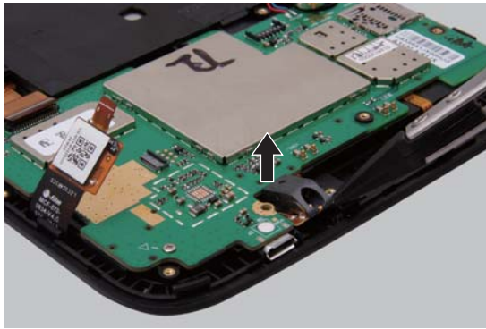
Figure 8. Removal steps of system board (continued)
