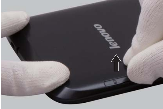
Figure 3. Removal steps of back cover
