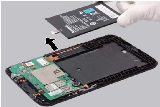
Figure 6. Removal steps of battery pack (continued)
