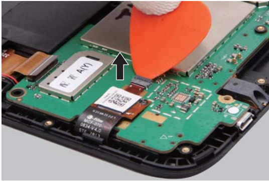
Figure 8. Removal steps of system board (continued)
