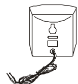
Speaker Wires (5 sets are attached to the back of the speakers)
