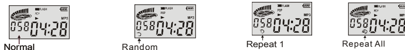
Fig. 3-6-2 Pressing the M-button a short time to select from the 4-mode playback sequence
