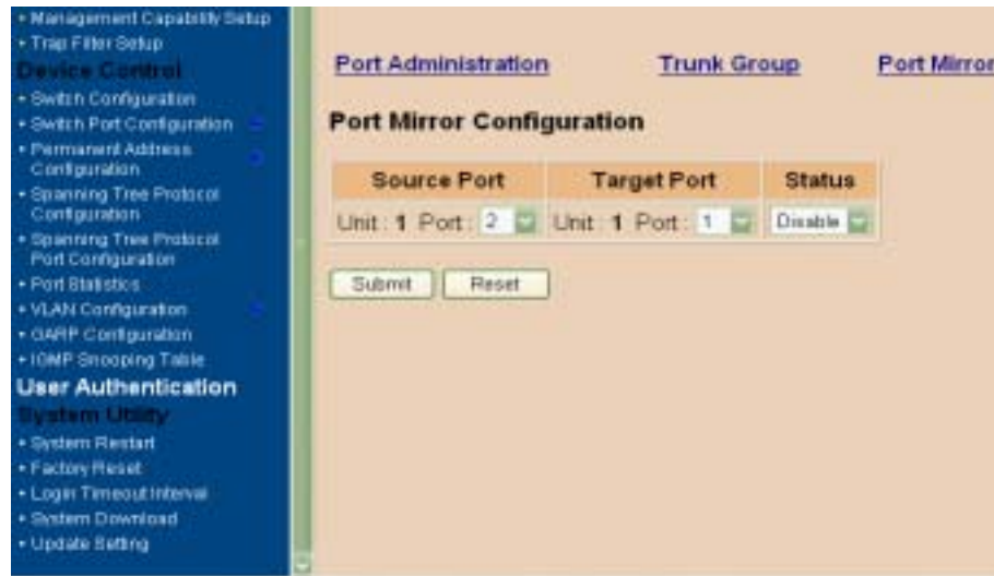
Figure 4-13. The Port Mirror in Switch Port Configuration Menu
