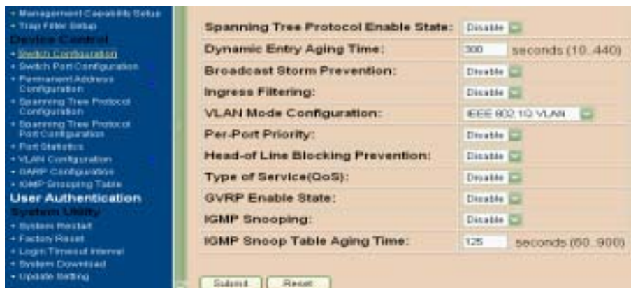
Figure 4-10. The Switch Configuration lower Menu
