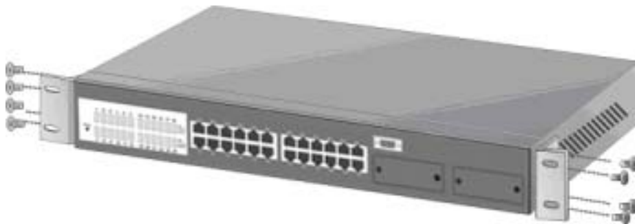
Figure 3-2. Attach mounting brackets with screws
