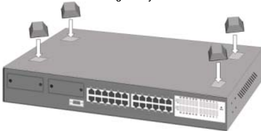
Figure 3-1. Attaching Rubber Feet to each corner on the bottom of the Switch
