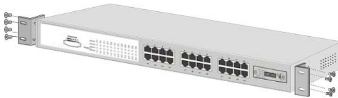
Figure 2-4. Attach mounting brackets with screws
