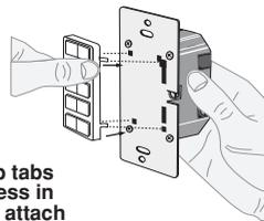
Line up tabs and press in side to attach
