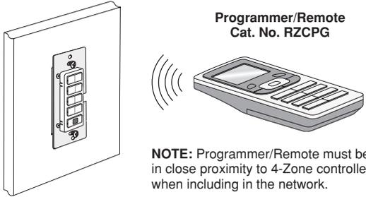
**NOTE:** Programmer/Remote must be in close proximity to 4-Zone controller when including in the network.
