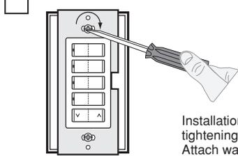
Installation may now be completed by tightening mounting screws into wall box. Attach wallplate.
