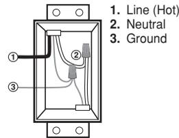
**Step 3** **Preparing and connecting wires:**
