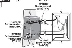
Terminal Label: Use Terminal for 3-Way or More Applications Only. For Single-Pole Applications, Do Not Remove This
