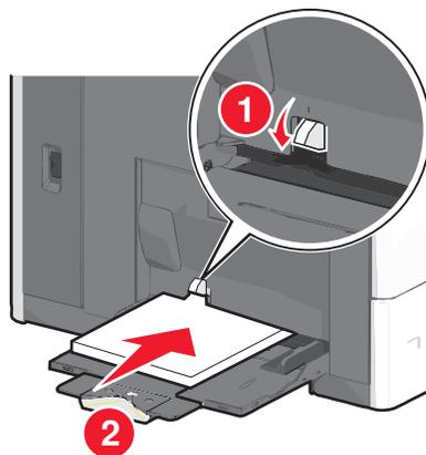
**Warning—Potential Damage:** Pulling the paper out, without pushing the paper pick tab first, may cause jams or the paper pick tab to break.
