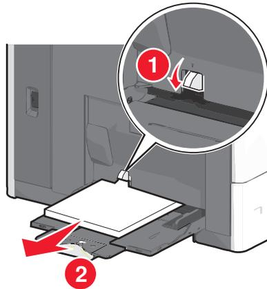
**Warning—Potential Damage:** Pulling the paper out, without pushing the paper pick tab first, may cause the paper pick tab to break.
