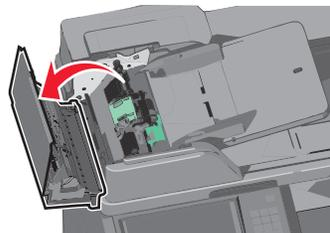
**4** Remove the pick roller assembly.
