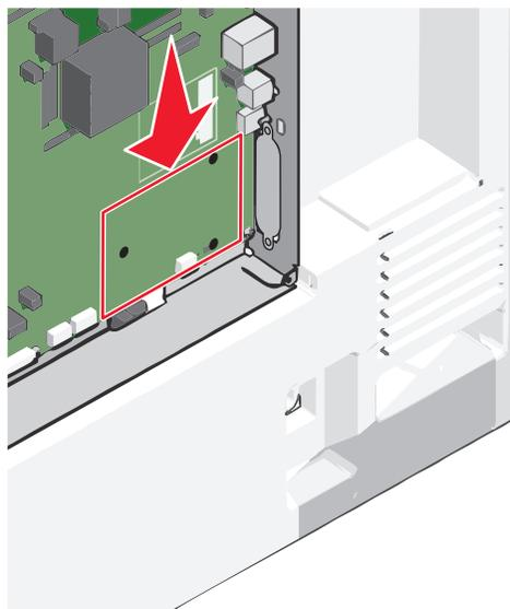
**4** Remove the printer hard disk.
