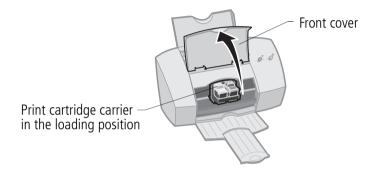
**3** Remove the old print cartridge. Store it in an air-tight container or dispose of it.
