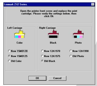
**8** If you installed a new cartridge, the Alignment dialog box displays. Follow the instructions on the Alignment screen to complete the cartridge installation. For help, see page 24.
