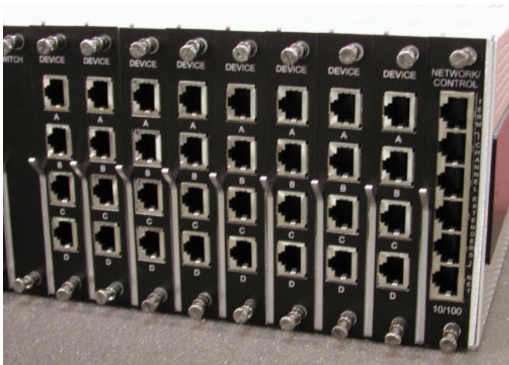
The NETWORK / CONTROL Card replaces the CONTROL card (far right slot) in 3200
