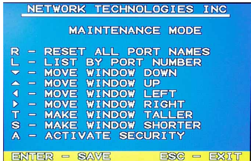
Figure 18- Maintenance Mode screen
