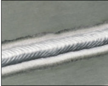
Pulse-On-Pulse™ on 3 mm Aluminum
