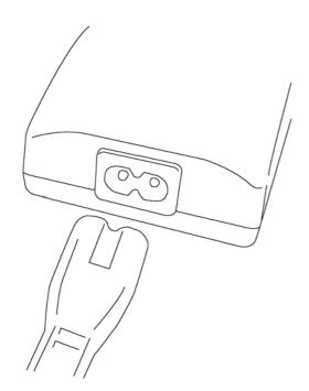
**3.** Plug the power cable into the power socket on the Ethernet Bridge.
