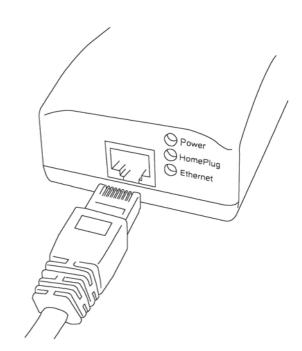
**1.** Plug the supplied Ethernet cable into the computer's RJ-45 network port.
