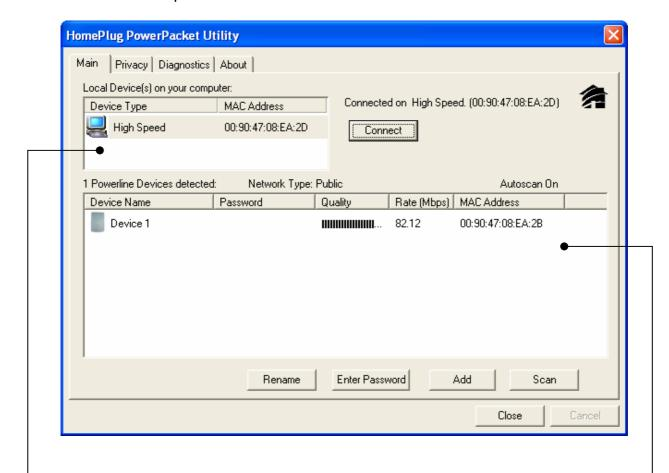
Shows the Powerline unit(s) currently connected to your PC. If you have more than one device, you can highlight it and click the **Connect** button to connect to it.
