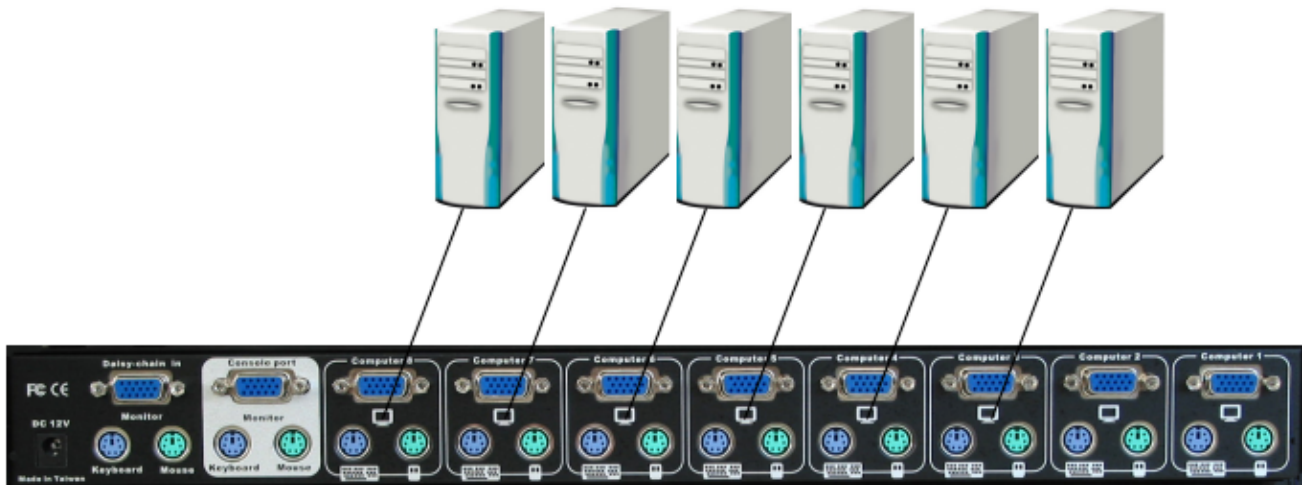
Computer connection (image shows CPU Switch P8 model)
