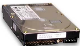
An 80 GB HDD is installed in the DVR
