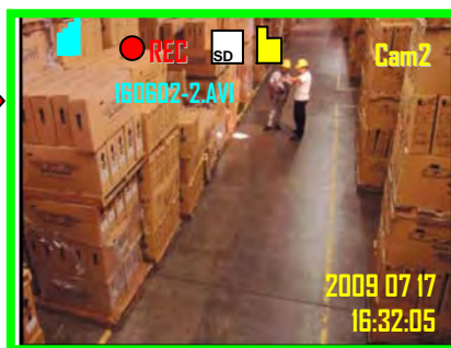
Camera 2 detects motion, so the system starts recording and camera 2 is displayed on-screen
