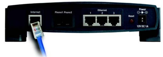
Figure 4-4: Connect the Cable/DSL Modem
