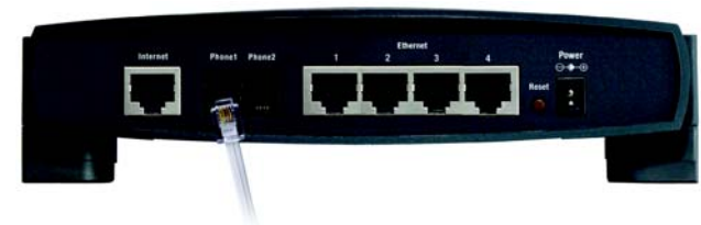
Figure 4-2: Connect a Telephone
