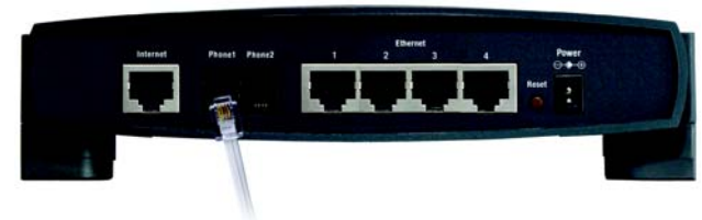
Figure 4-7: Connect a Telephone
