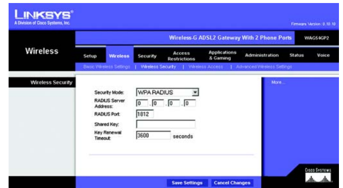
Figure 4-18: Wireless Tab - Wireless Security (WPA RADIUS)
