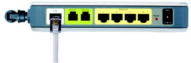
Figure 3-2: Connecting your ADSL line
