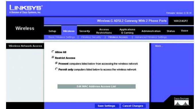
Figure 4-20: Wireless Tab - Wireless Network Access
