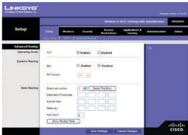
Setup > Advanced Routing
