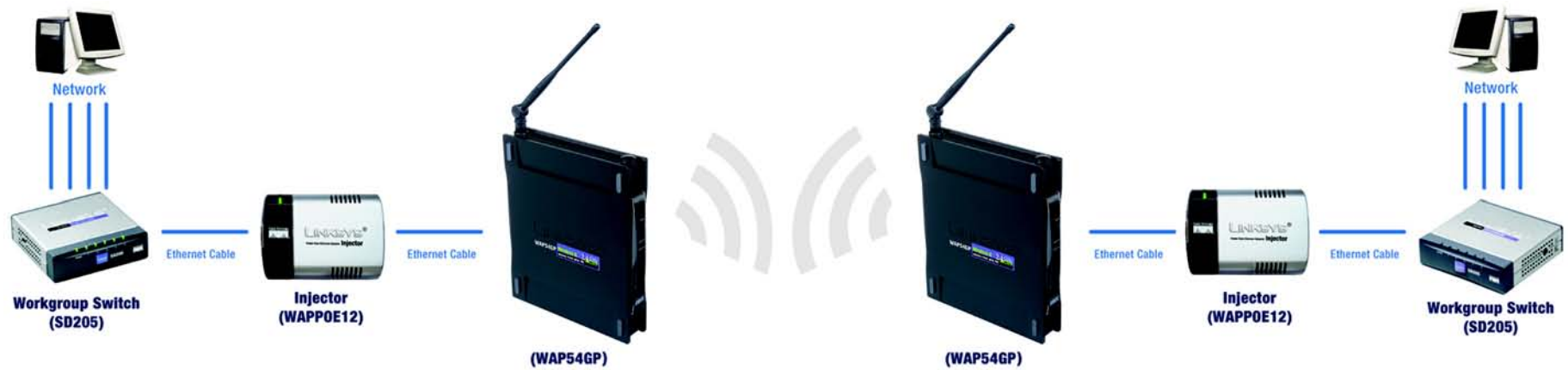
Figure 5-15: Wireless Bridge Diagram
