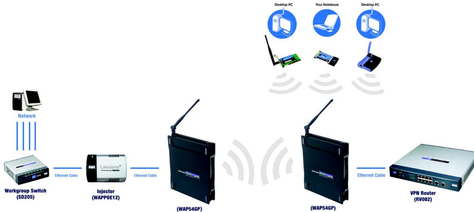
Figure 5-13: Wireless Repeater Diagram
