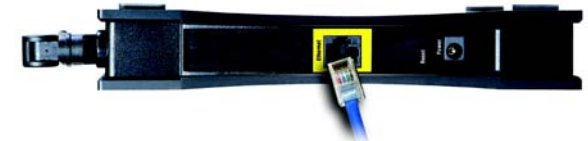
Figure 4-1: Connect the Ethernet Network Cable
