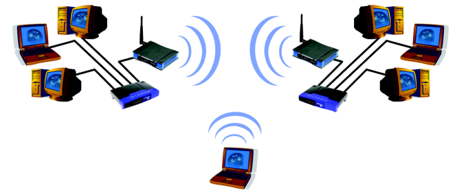
Figure 2-3: Network Using Wireless Bridging
