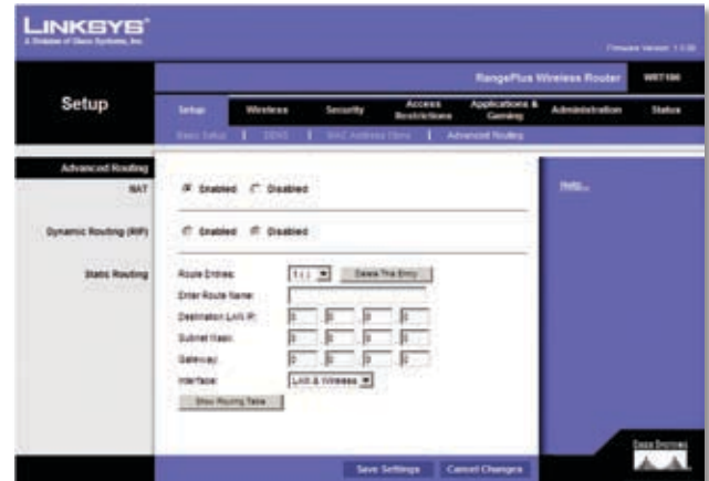
Setup > Advanced Routing
