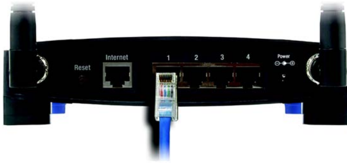
Figure 4-6: Connecting Your Network Devices
