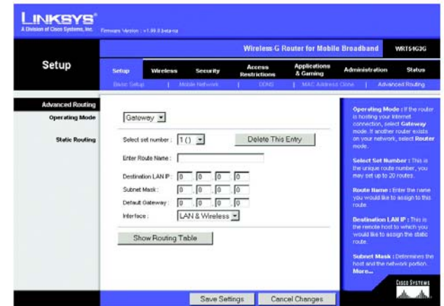
Figure 5-16: Setup Tab - Advanced Routing (Gateway)
