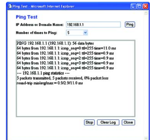
Figure 5-43: The Ping Test
