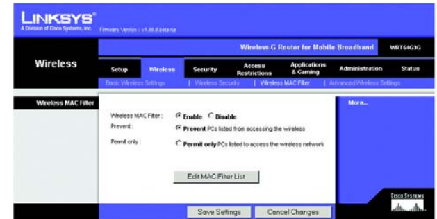
Figure 5-27: Wireless Tab - Wireless MAC Filter
