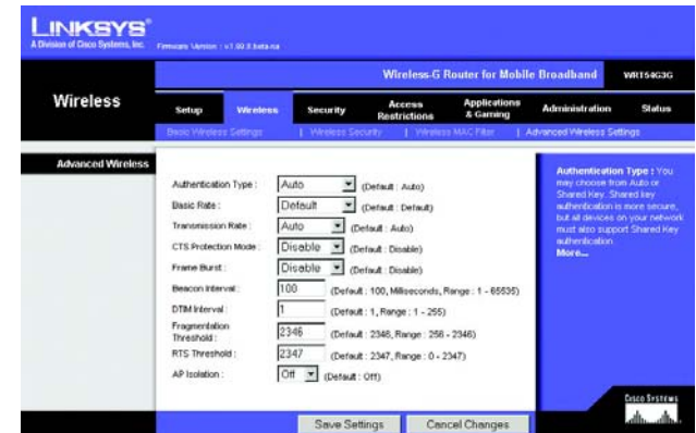
Figure 5-29: Wireless Tab - Advanced Wireless Settings
