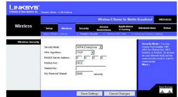
Figure 5-23: Wireless Tab - Wireless Security (WPA Enterprise - TKIP)
