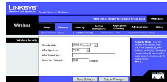
Figure 5-20: Wireless Tab - Wireless Security (WPA Personal - TKIP)
