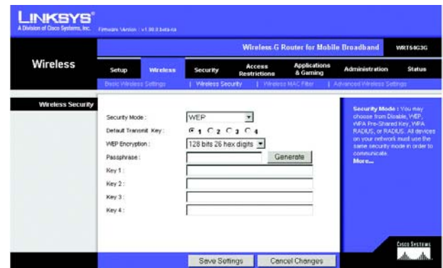
Figure 5-26: Wireless Tab - Wireless Security (WEP)
