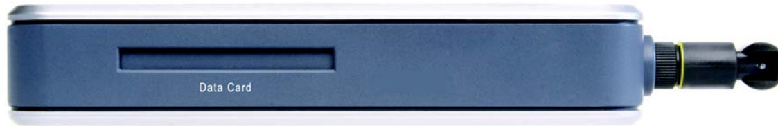
Figure 3-4: The Router's Data Card Slot
