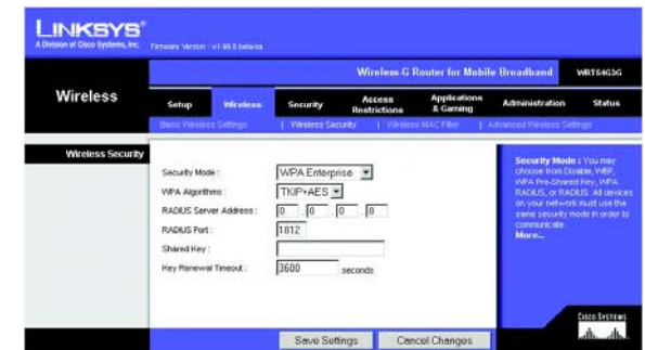
Figure 5-24: Wireless Tab - Wireless Security (WPA Enterprise - AES)
