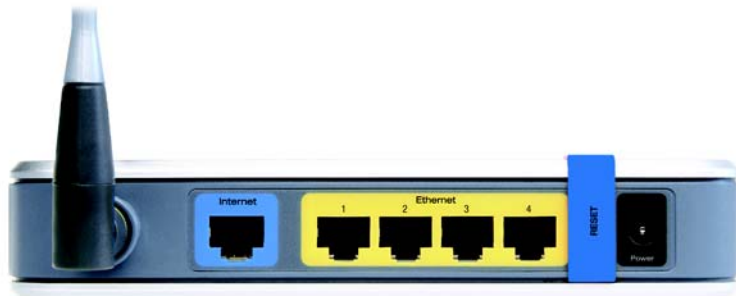
Figure 3-1: The Router's Ports
