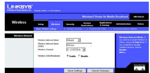
Figure 5-18: Wireless Tab - Basic Wireless Settings
