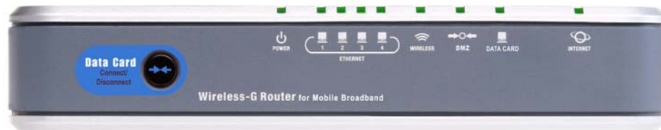
Figure 3-3: The Router's LEDs
