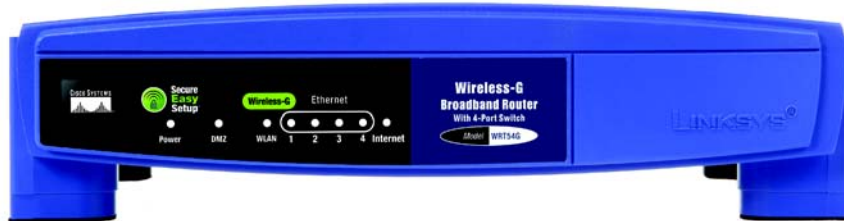
Figure 3-2: The Router's Front Panel
