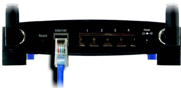
Figure 4-5: Connecting Another Router
