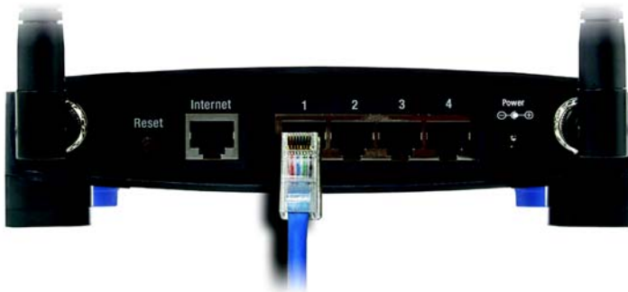
Figure 4-2: Connecting Your Network Devices
