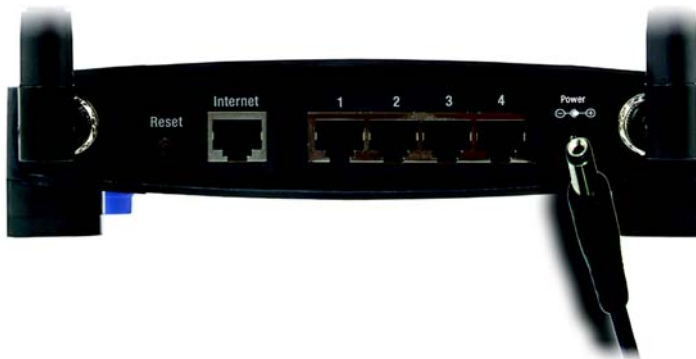
Figure 4-3: Connecting the Power
