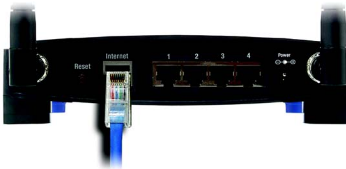
Figure 4-1: Connecting Your Internet Connection
