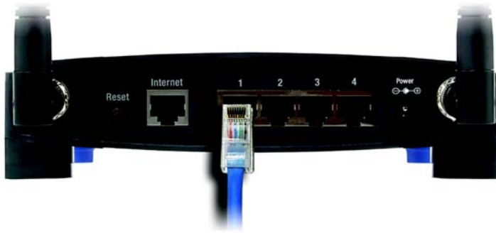
Figure 4-6: Connecting Your Network Devices
