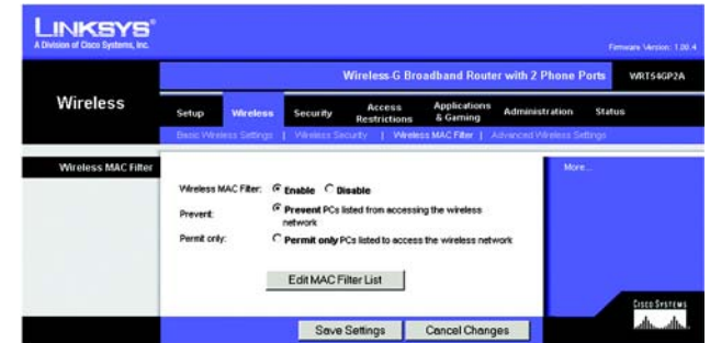
Figure 5-15: Wireless Tab - Wireless MAC Filter
