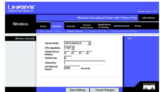
Figure 5-12: Wireless Tab - Wireless Security (WPA RADIUS)
