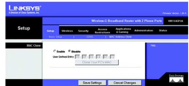
Figure 5-9: Setup Tab - MAC Address Clone
