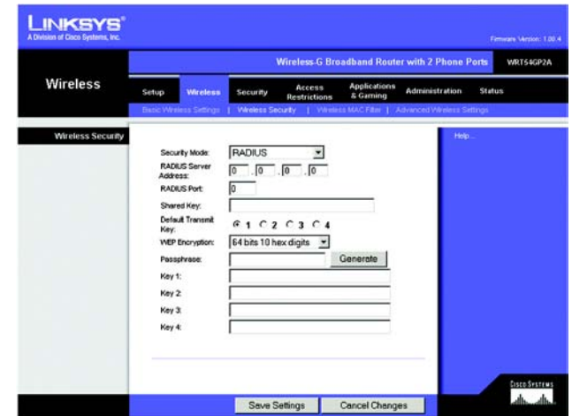
Figure 5-13: Wireless Tab - Wireless Security (RADIUS)
