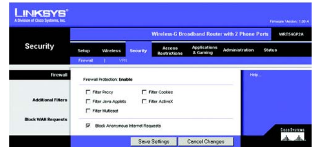
Figure 5-19: Security Tab - Firewall
