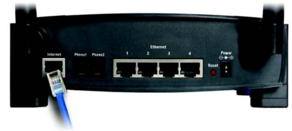
Figure 4-6: Connect the Broadband Modem
