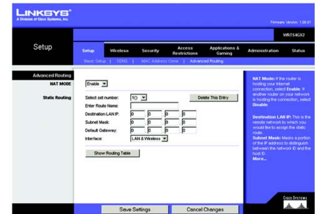
Figure 5-15: Setup Tab - Advanced Routing - NAT Mode
