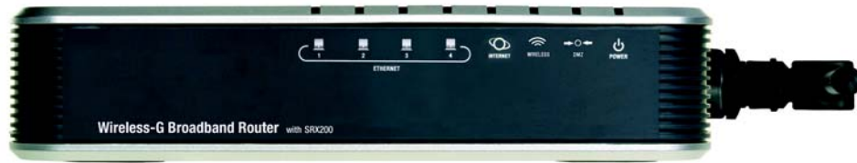
Figure 3-2: The Router's LEDs
