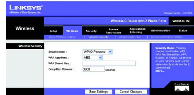
Figure 5-20: Wireless Tab - Wireless Security (WPA2 Personal)
