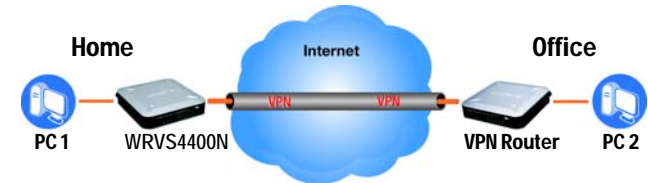
Figure 3-1: VPN Router to VPN Router
