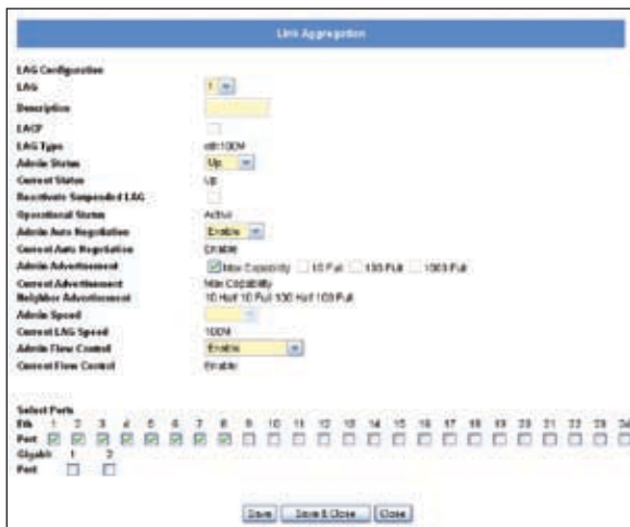
Port Management > Link Aggregation > Detail
