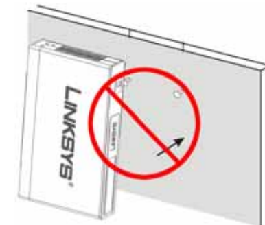
Figure 3-5: Incorrect Wall-Mount Orientation (Vertical)
