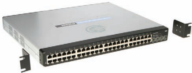
Attach the Brackets to the Switch
