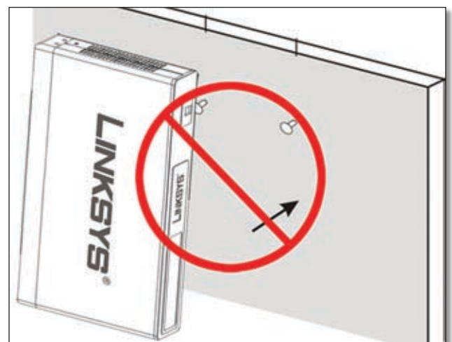
Incorrect Wall-Mount Orientation (Vertical)
