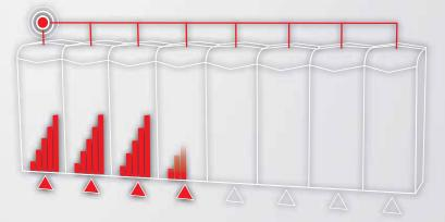
Cascading continues as additional boilers fire in sequence, until all units are in operation or demand is satisfied. When demand drops, the patented cascading process reverses, with the precision, control and performance you expect from Lochinvar.
