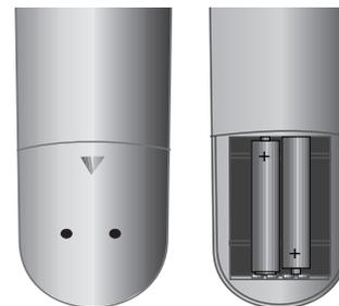
To insert or change the batteries, press on the imprinted arrow. Slide off and remove the battery compartment cover. Insert alkaline-manganese LR 03 (AAA) type batteries and make sure the + and - poles are aligned correctly. Then, replace the cover.
