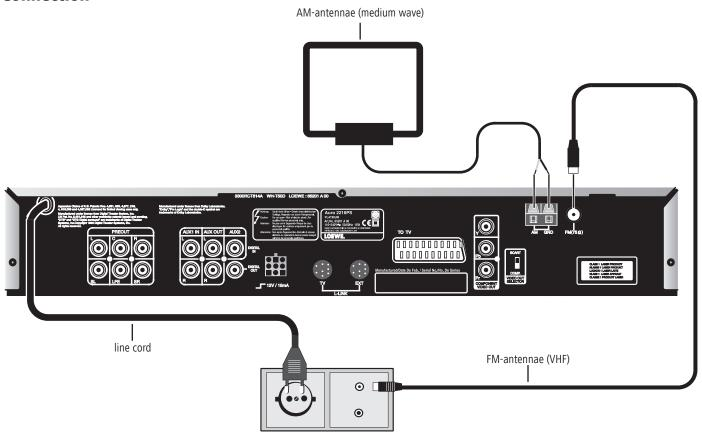
**Attention**: All the devices involved must be disconnected from the mains when you are connecting the cables.
