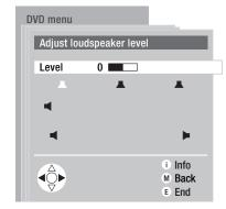
You hear a noise in turn from every single loudspeaker starting with the front left speaker. The speaker is highlighted in white in the overview (see the figure) whilst the noise is being emitted from it. You can reduce or increase the volume of this loudspeaker whilst the noise is being emitted from it. Listen to all the speakers once first. The perceived volume should have the same intensity from all speakers.
