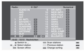
The FM-Radio station table holds a maximum of 36 stations. In our example, 29 stations have been found in the initial installation and entered in the station table.
