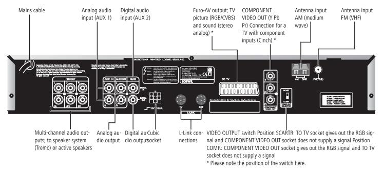
Caution: Do not touch the inner pins of connection sockets on the rear panel. Electrostatic discharge may cause permanent damage to the unit.
