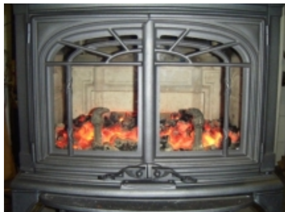
Let the stove burn with the bypass and air control open for about 45 minutes to establish a good coal bed (3" to 4").
