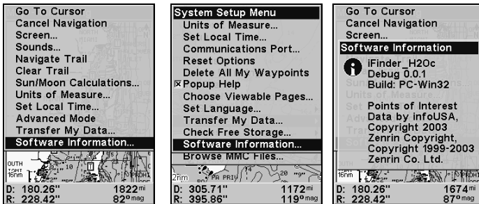
Software Info command in Easy Mode (left). Advanced mode (center). The Software Info screen (right).
