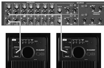
Control Room Router (Balanced TRS to Balanced XLR)
